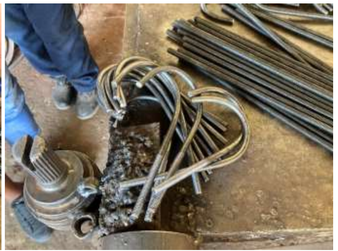
Above: the creation of the 1600 fastening hooks. Below: the corrugated sheet metal for the new roof.
